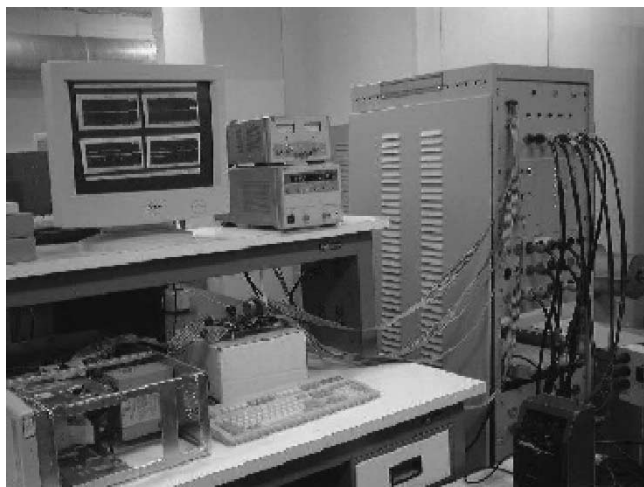
Fig. 2. StatCom rack with graphical user interface.
