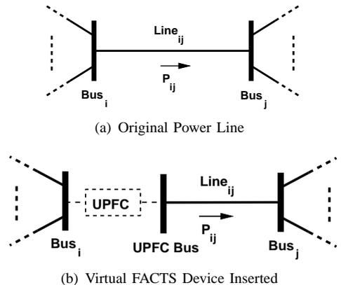
Fig. 1. Original Line Model and Modifications for simulated UPFC
