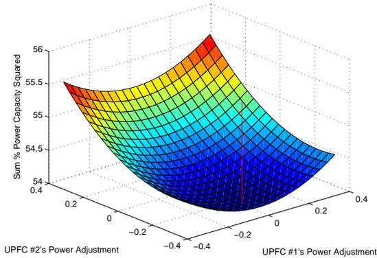
(a) Example of the effects on the objective function of UPFCs installed on lines 27 and 110
