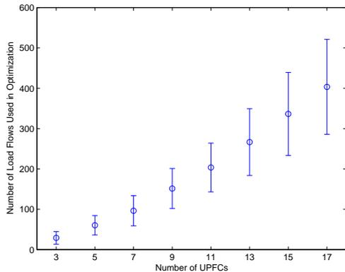
Fig. 3. Number of Load Flow calls used per optimization vs. number of UPFCs; central point is the mean and the error bars include the 95 percentile of 100 random samples
